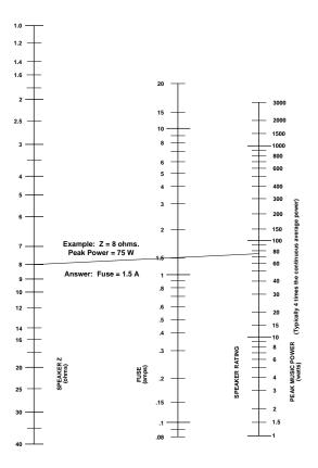
Fig. 2.4 Loudspeaker Fuse Nomograph
