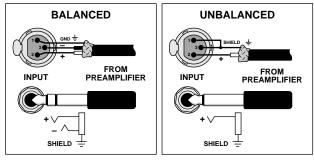
Fig. 2.2 CSL Input Wiring
