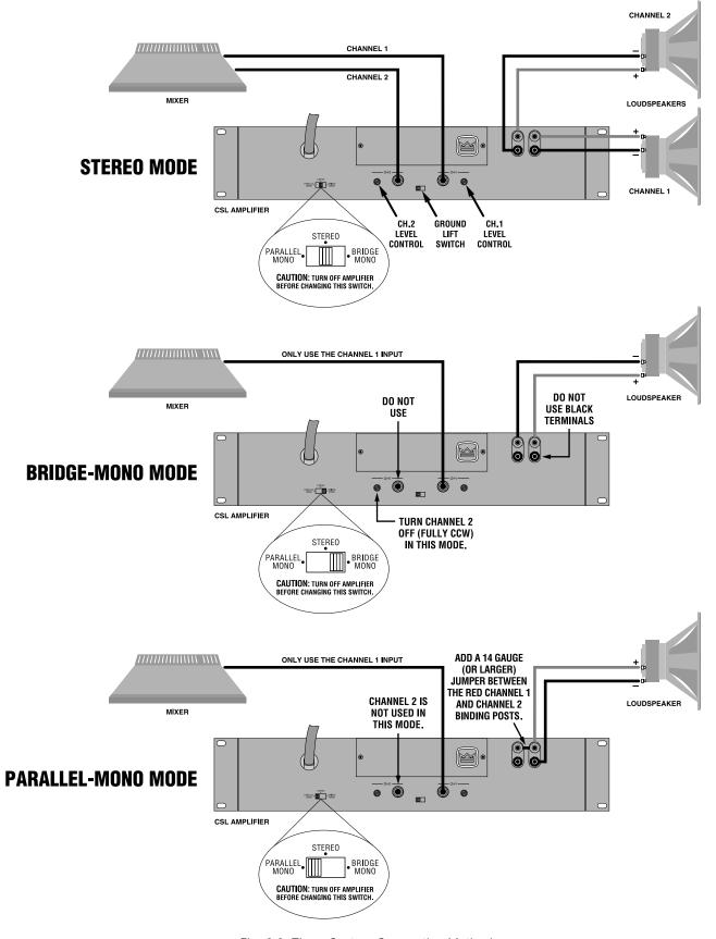
Fig. 2.3 Three System Connection Methods
