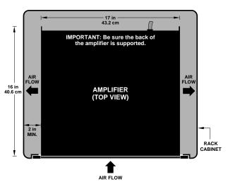
Fig. 2.1 Do NOT Block Air Flow
